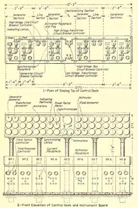
Fig. 235.—Plan of face of desk and front elevation of control desk and instrument board.
